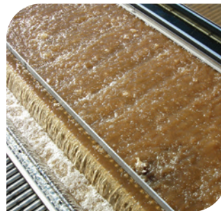
Agitation shown. Water level usually lowered to avoid carryover.
